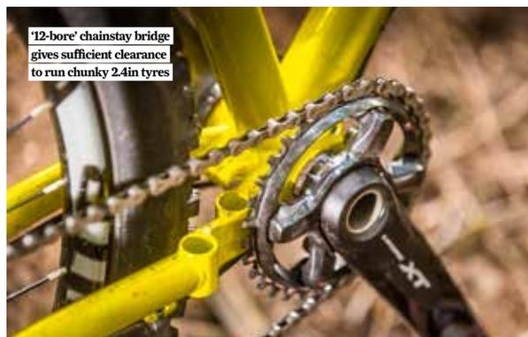
'12-bore' chainstay bridge gives sufficient clearance to run chunky 2.4in tyres
